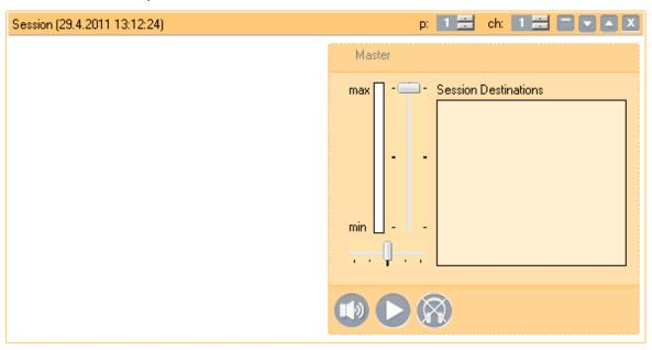
a. Using Drag & Drop assign the destination to the session. Simple move the highlighted speaker over the Master fader of the particular session.
